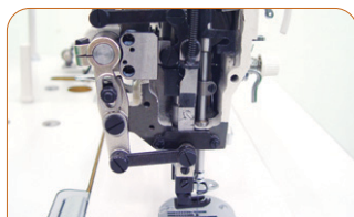
Realization of Upper/Lower Feed Mechanism
